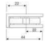
GW-725 Straight edge 90° Double side glass partition brace ★ Materials: Refined Stainless steel ★ Finish: Mirror
